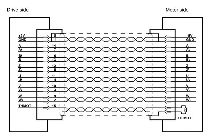
A, A/, B, B/, Z, Z/, U, U/, V, V/, W, W/, 5V, GND and Th.mot. To work properly and with respect of the trigonometric sense of rotation, B and B/ must be crossed.
