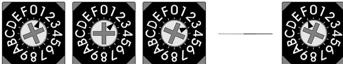
The axis selector defines the axis number of the drive, from address 1 to 15. The drive will reply to RS485 messages sent to the corresponding address (Axis selector on 5  $\Rightarrow$  drive reply to messages sent to address Nr. 5).
