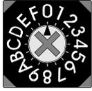
The axis selector must be on « 0 », the drive replies to RS232 messages sent to address Nr.1.
