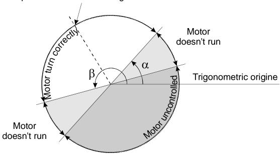
The optimal value of « Resolver shift angle » is given by :
