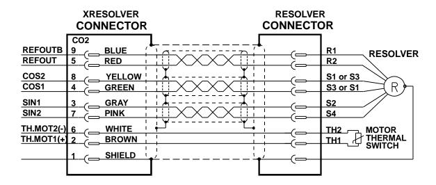
Figure 2 - Resolver and motor thermal switch wiring
