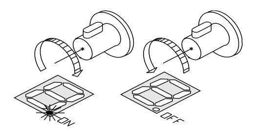
If the decimal point lights up during anti-clockwise rotation, wires S1 (COS1) and S3 (COS2) of resolver connector must be inverted (see section 1.3.1 of chapter D).
